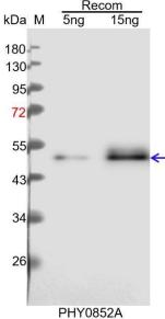
Recom: 5 ng and 15 ng recombinant protein containing the peptide for immunization and having a molecular mass of 50 kDa. Electrophoresis: 12% SDS-PAGE. **Transfer:** blotting to NC (nitrocellulose) membrane for 1 h. **Blocking:** 5% skim milk at RT or 4°C for 1 h. **Primary antibody:** 1:1000 dilution overnight at 4°C. Secondary antibody: 1:10000 dilution using Goat Anti-Rabbit IgG H&L (HRP) (Cat# PHY6000). Detection: using chemiluminescence substrate and image were captured with CCD camera.
