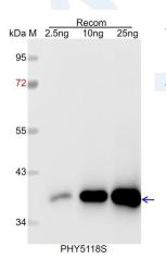
Recom: 2.5 ng, 10 ng and 25 ng recombinant protein containing the peptide for immunization and having a molecular mass of 38 kDa. **Electrophoresis:** 12% SDS-PAGE **Transfer:** blotting to NC (nitrocellulose) membrane for 1 h. **Blocking:** 5% skim milk at RT or 4°C for 1 h.
